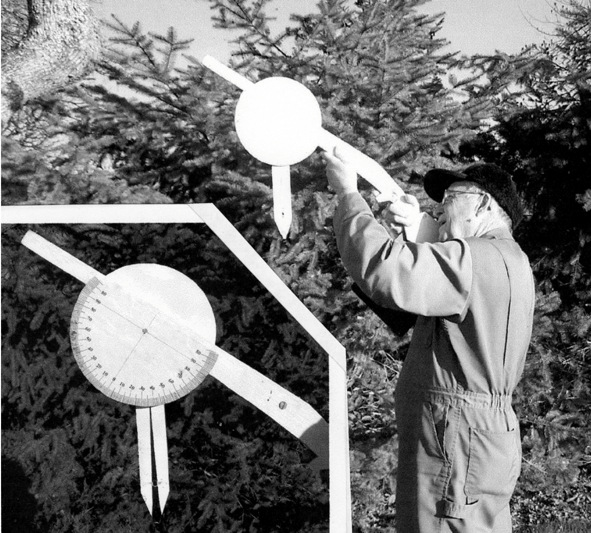
Figure 32 Slope gauge with weighted pointer reads 36 degrees. While using surveyor's equipment could make more precise measurements, this simple tool easily measured within 1 degree, which is adequate for this study.
